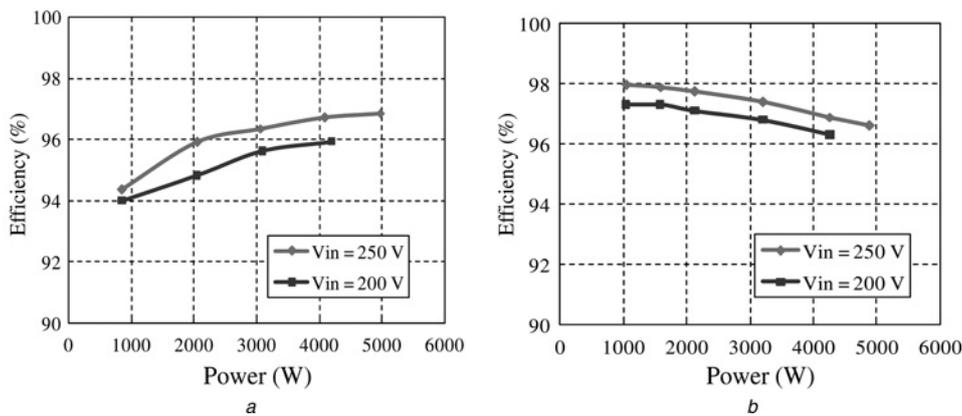
**Fig. 10** Efficiency of the dc/dc converter at a case temperature of 140°C using SiC-VJFET devices from two different device lots
