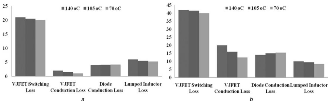
Fig. 7 Losses (in watts) of a single converter module (in boost mode) at an input voltage of 250 V for varying case temperatures and at
