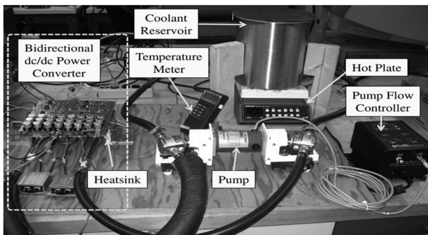
Fig. 6 Experimental setup for evaluating the performance of the dc/dc converter using high-temperature inlet coolant
