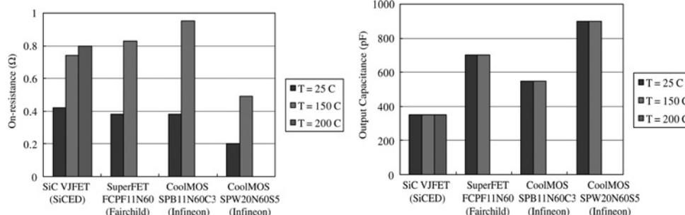
**Fig. 2** Comparison of the on-resistances and output capacitances of SiC VJFET with state-of-the-art Si MOSFETs
