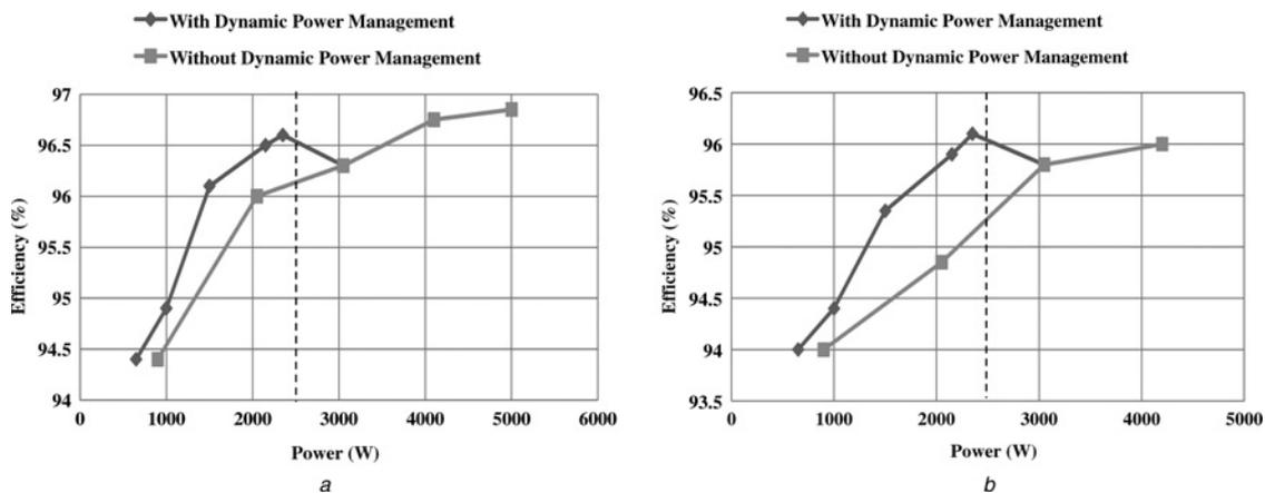
**Fig. 11** Variation of efficiency of the dc/dc converter at 140°C for input voltages of a) 250 V and b) 200 V, respectively
