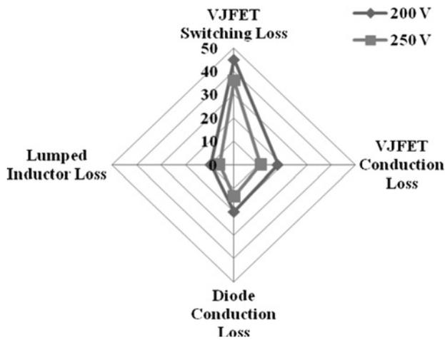
**Fig. 9** Breakup (in watts) of key loss components for each dc/dc converter module operating at full load for two input voltages
