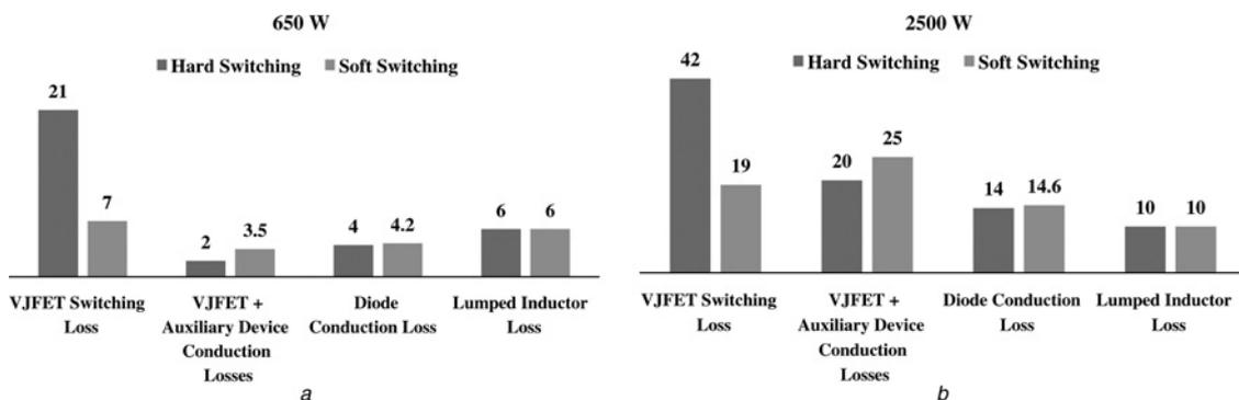
Fig. 14 Comparison of the losses (in watts) of the hard-switched and soft-switched converters at
