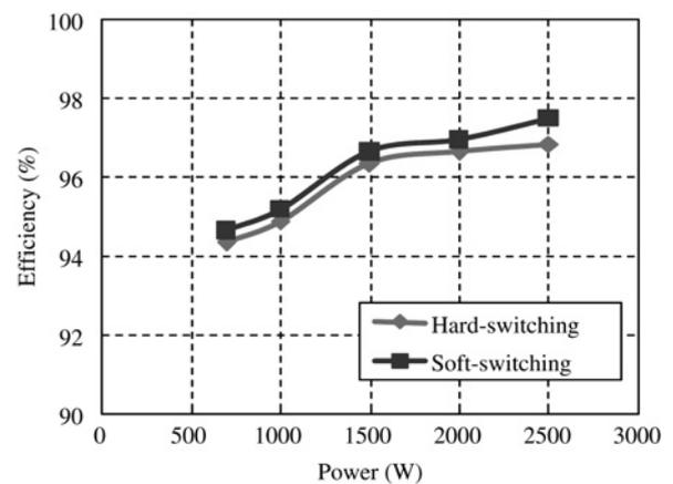
Fig. 13 Converter-module efficiencies against output power at a case temperature of 140°C and for  $V_{in} = 250$  V
