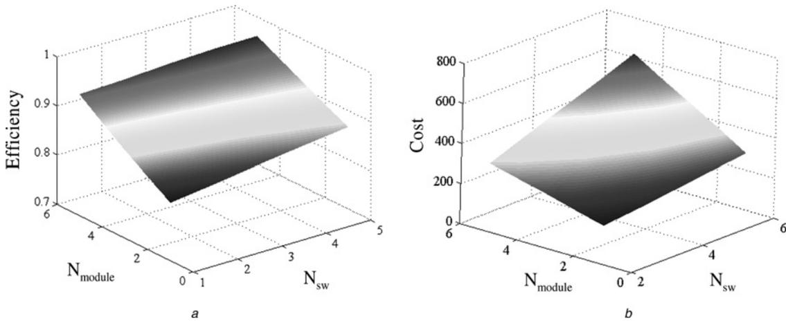
**Fig. 4** Variation of the dc/dc multiphase converter with variations of the number of converter modules ( $N_{module}$ ) and the number of SiC VJFETs ( $N_{sw}$ ) connected in parallel in each converter module
