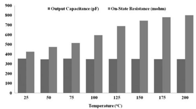
Fig. 8 Variations of the output capacitance and on-state resistance of a SiC VJFET with increasing case temperature
