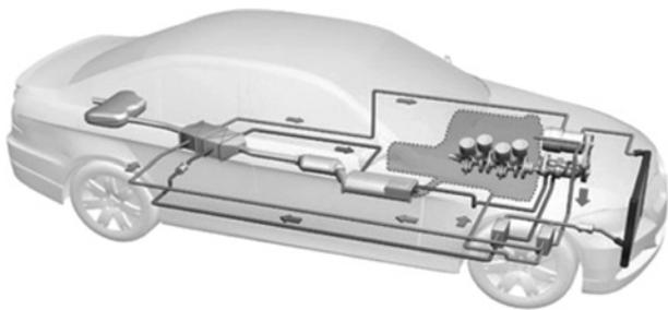
**Fig. 1** Illustration of two-coolant system [14] in conventional PHEV/HEV that increases system cost and complexity
