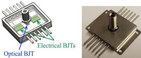
Fig. 3. Fabricated Darlingon OTPT in one package.
