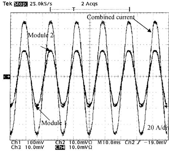
Fig. 16. Input current of the parallel modules and the total current in that phase.
