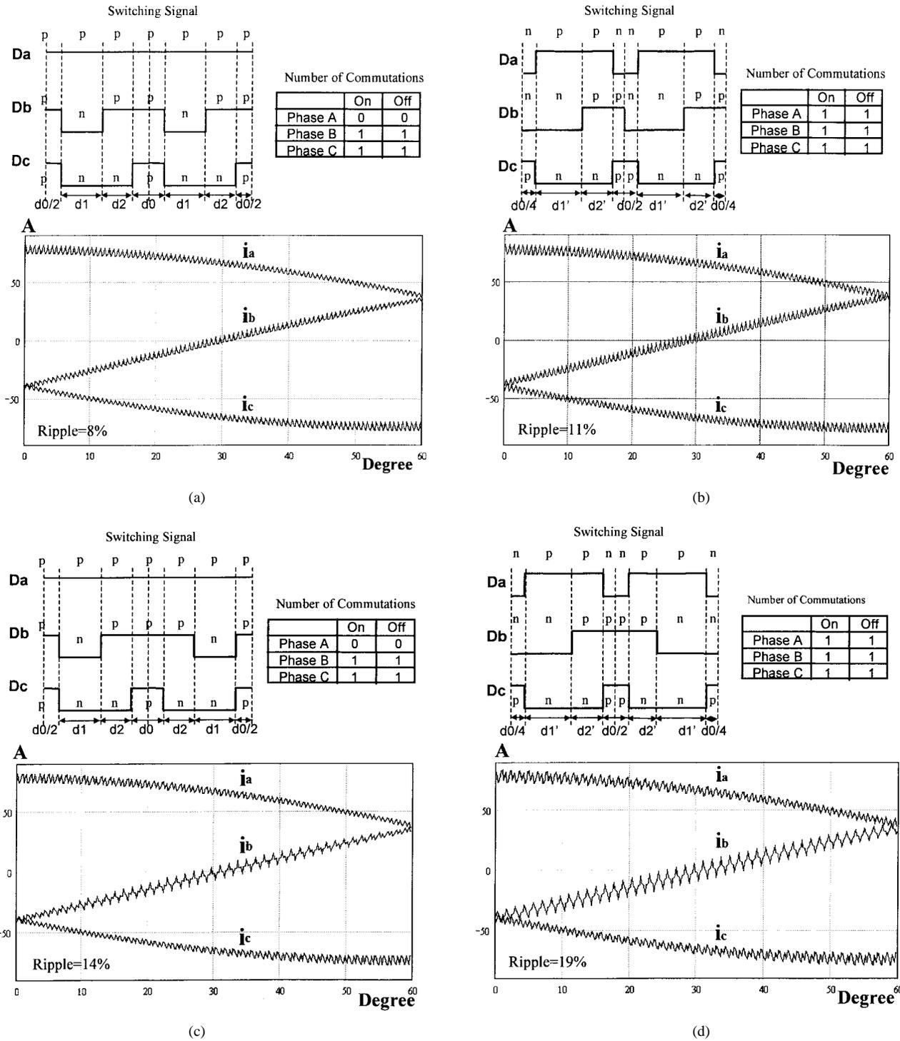
Fig. 21. The comparisons between SVM's in commutation times and current ripples. (a) and (b) Asymmetrical 60° clamping SVM and the SVM without using zero vectors. (c) and (d) Symmetrical operation.
