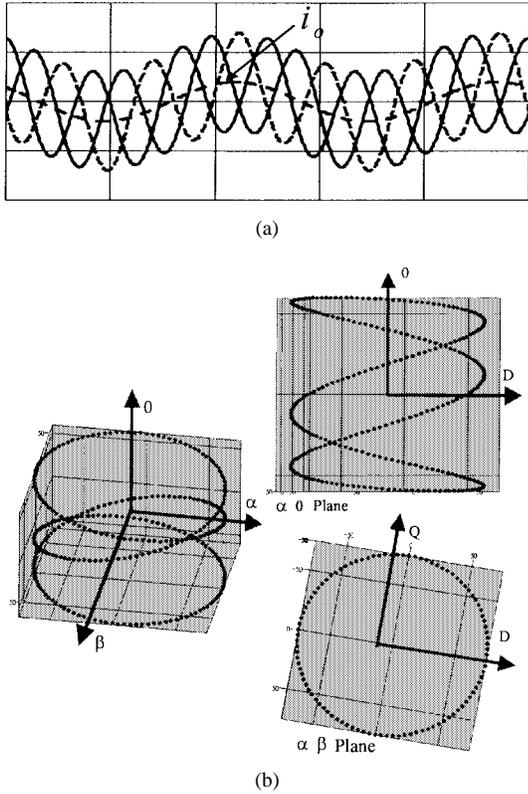
Fig. 10. (a) The effect of the pure zero-sequence current in time frame. (b) Three-dimensional (3-D) view of the three-phase current with a zero-sequence current in the rotating frame.
