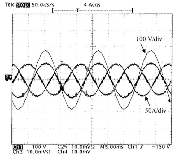
Fig. 15. Input voltage and current waveform in single-module operation.
