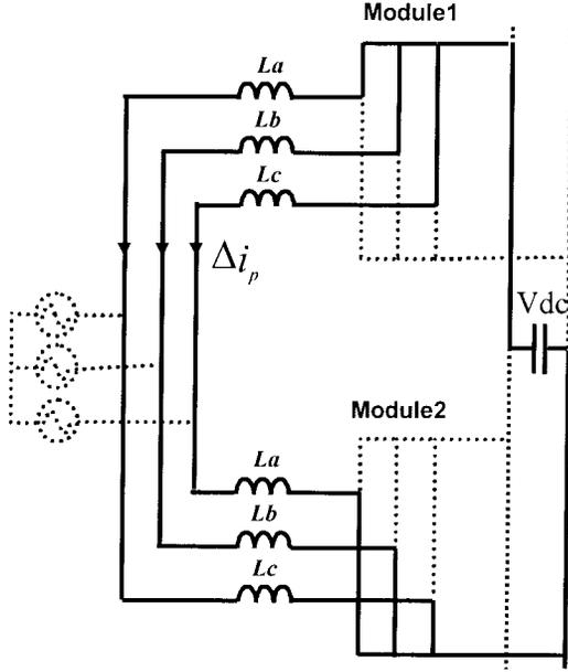
Fig. 8. The path of the pure zero-sequence current.
