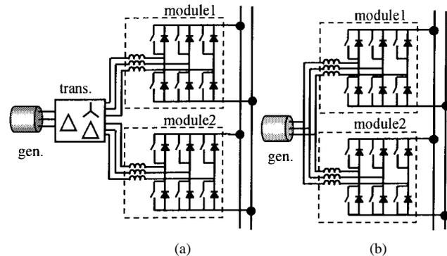
Fig. 1. Typical configurations of parallel rectifier on a single source (a) with a phase-shifted transformer and (b) with an interleaved PWM.
