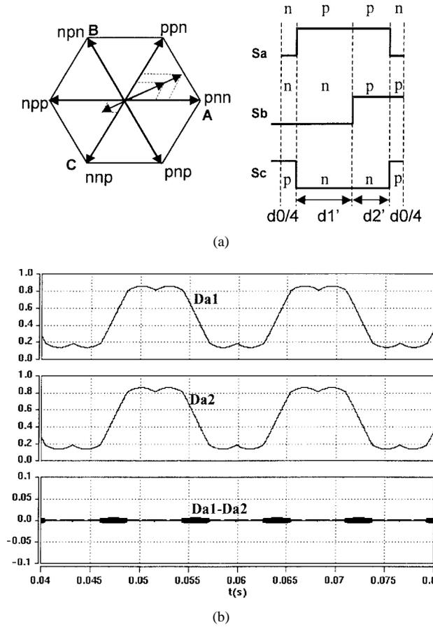
Fig. 12. (a) The proposed SVM for parallel operation without using zero vectors. (b) The averaged phase duty cycles and the difference between them.
