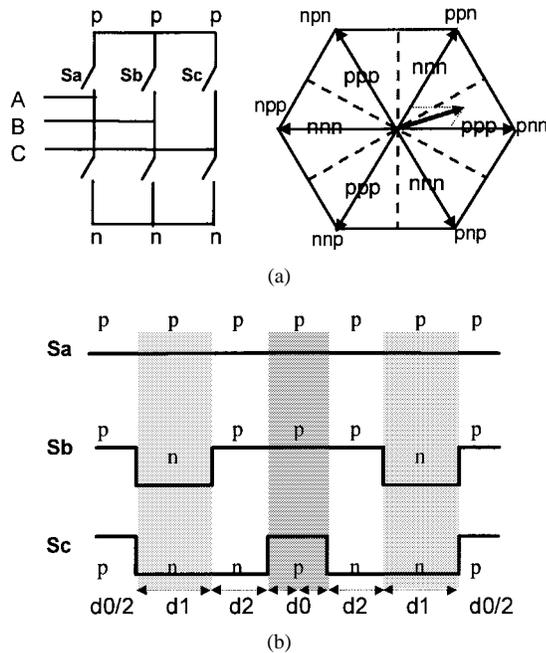
Fig. 4. The 60° clamped SVM.
