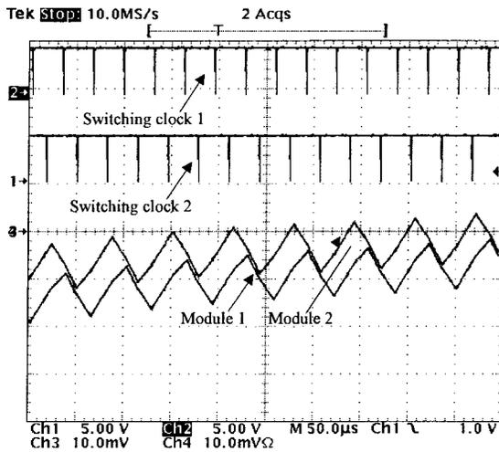
Fig. 17. Interleaved switching clock and the resulting current waveform.
