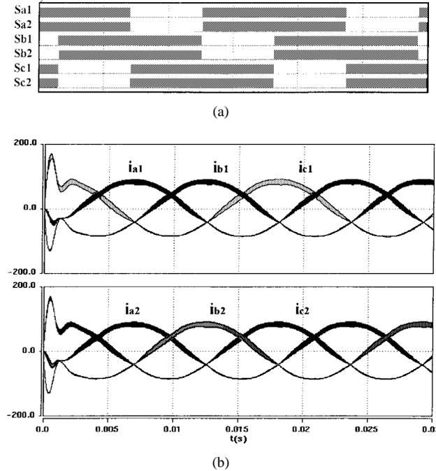
Fig. 11. (a) The gate signals of the top switches of the paralleled module with hysteresis control. (b) The three-phase input current of the paralleled module.
