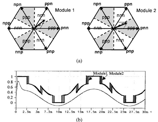
Fig. 7. (a) The position of reference vectors when passing the discontinuous point. (b) The duty-cycle difference of the interleaved discontinuous SVM.
