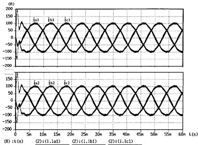
Fig. 13. Three-phase input current with the proposed SVM.
