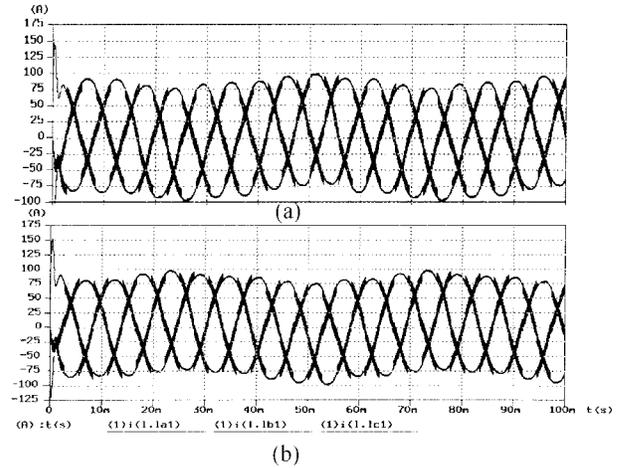
Fig. 3. Input current waveform of the paralleled modules.
