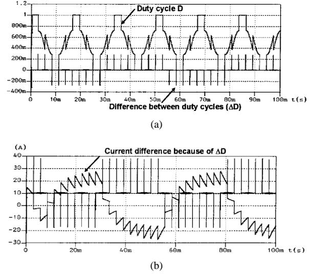
Fig. 9. Beat-frequency oscillation of the zero-sequence current.
