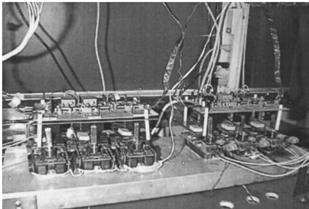
Fig. 14. Paralleled three-phase system based on the modular concept.
