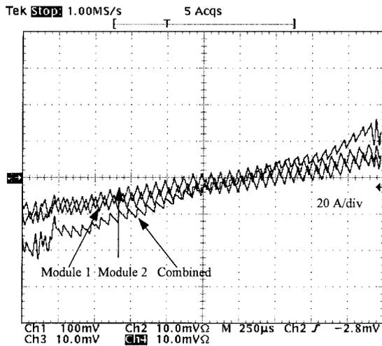
Fig. 18. Extended view of the current waveforms.
